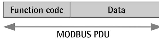
The mapping of Modbus protocol on a specific bus or network introduces some additional fields on the Protocol Data Unit. The client that initiates a Modbus transaction builds the Modbus PDU, and then adds fields in order to build the appropriate communication PDU.
